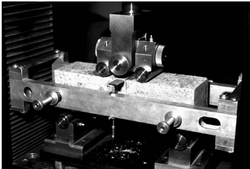
FIG. 1 Arrangement to Obtain Net Deflection by Using Two Transducers Mounted on Rectangular Jig Clamped to Specimen Directly Above Supports
